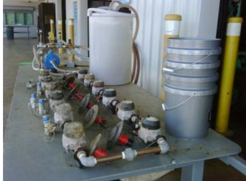
Pilot plant consumption testing as a water meter upgrade research tool
