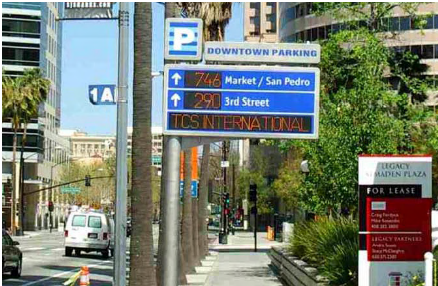
Typical Small Dynamic Vehicular Wayfinding Sign
