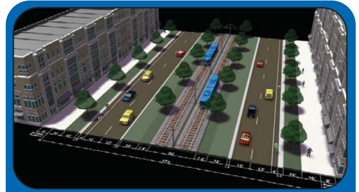
University City Area Plan streetscape rendering with sidewalks, planting strips, bicycle lanes, and light rail transit
