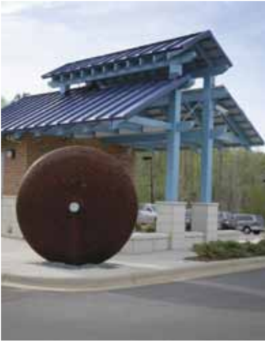
Corten steel responds to weather by rusting to a natural stopping point.
