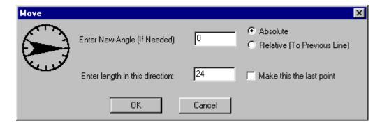
Type 24 in the box and press **ENTER**. The line created automatically cut the large area in two and divided the line into the appropriate dimensions. The drawing should now look like this:
