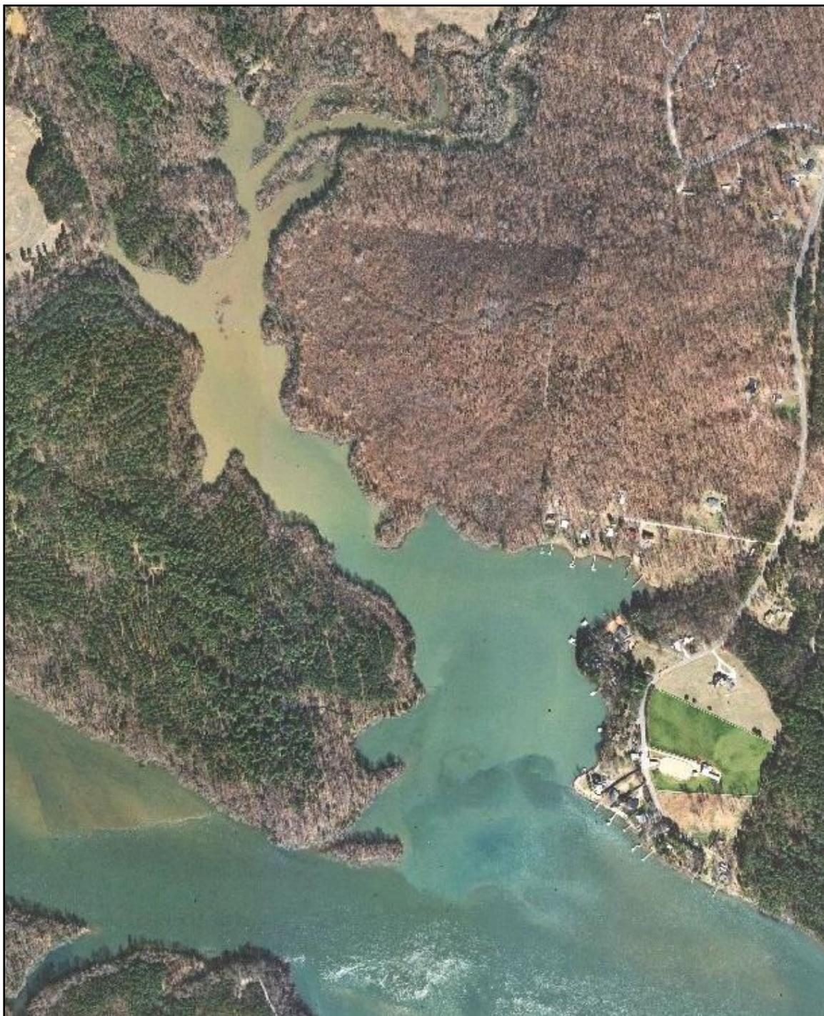
**Figure 11: Sediment Transported Down McDowell Creek into Mountain Island Lake.**
