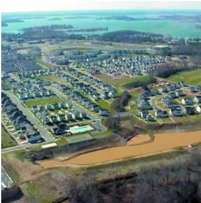
Increased impervious cover leads to increased non-point source pollution that can be controlled using wet ponds.
