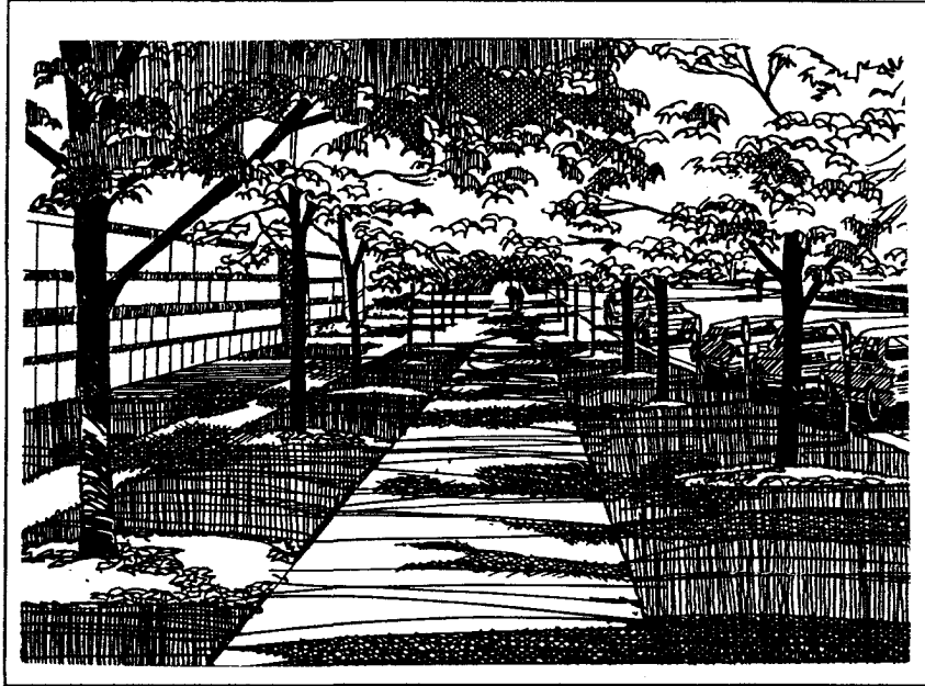
Street trees in wide planting strips create an inviting pedestrian environment by providing shade and buffering the pedestrian from busy streets.
