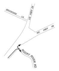
The intersection will be constructed to allow right turns only and prohibit left turns and/or through movement. While this alternative limits access to Rocky River Road, it has less potential for congestion on N.C. 49 and U.S. 29 than a full access signal.
