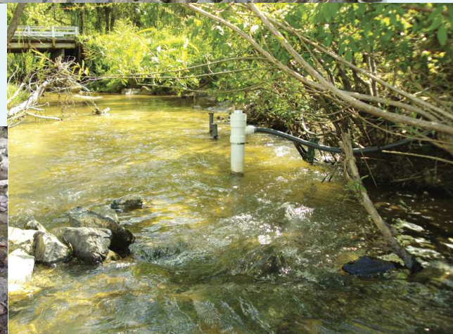
above In-stream grab sample collection below Qualitative stream biology sample collection at right Continuous automated in-stream monitoring
