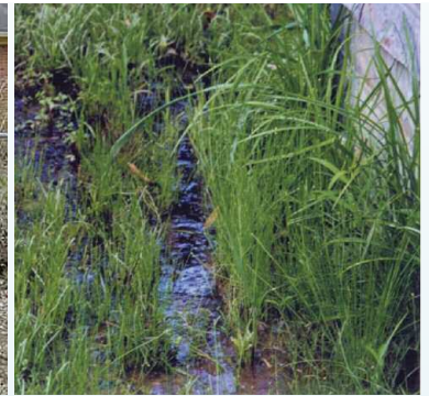
System failure: sewage surfacing on the ground and running along the property line.
