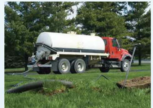
Septic tank pump truck
