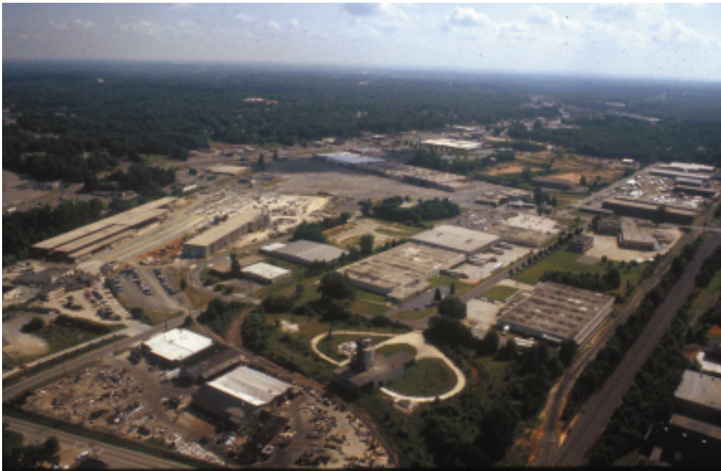
This area of the Little Sugar Creek watershed (N. Tryon and Sugar Creek Rd.) Has among the highest percentage of impervious cover in the county.
