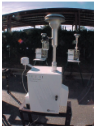
Typical PM 2.5 particulate monitor.
