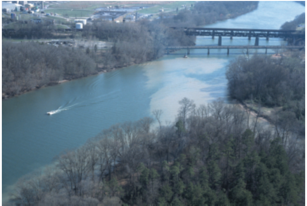
Plume of sediment from Dutchmans Creek entering upper Lake Wylie after a storm event shows the influence of tributaries on the water quality of the main stem of the Catawba.
