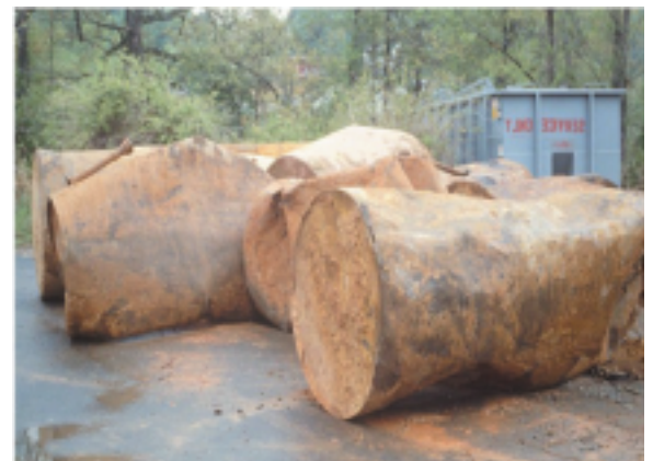
Steel underground storage tanks corrode with time.
