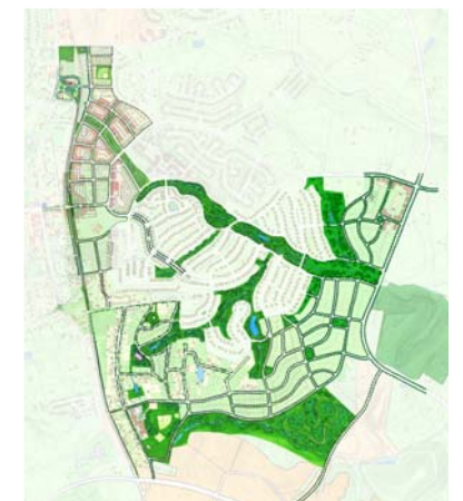
Frameworks Diagram showing improvements to open space network through a system of parkways and trails, including formalized and more natural open spaces.
