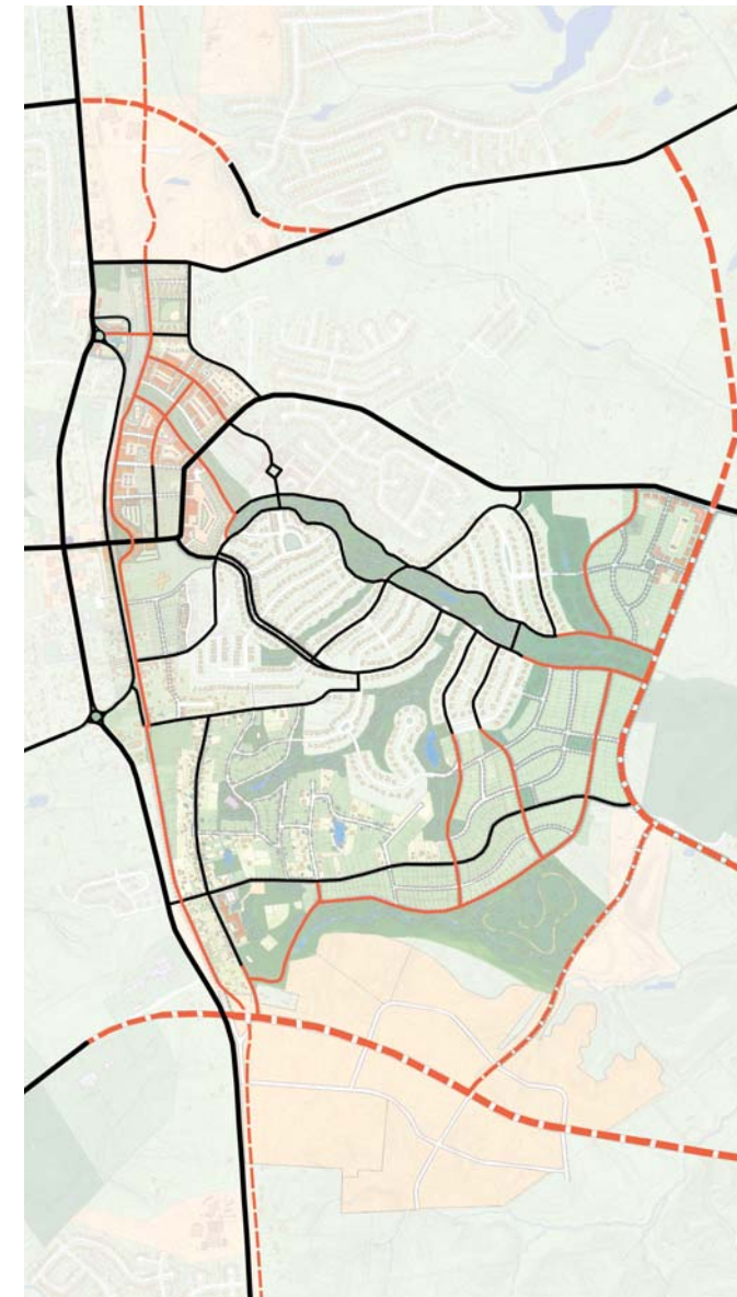
LOCAL CONNECTORS Diagram illustrating the pattern of secondary connectors, in addition to primary collectors shown previously. Secondary connectors provide links between the thoroughfares and local destinations.
