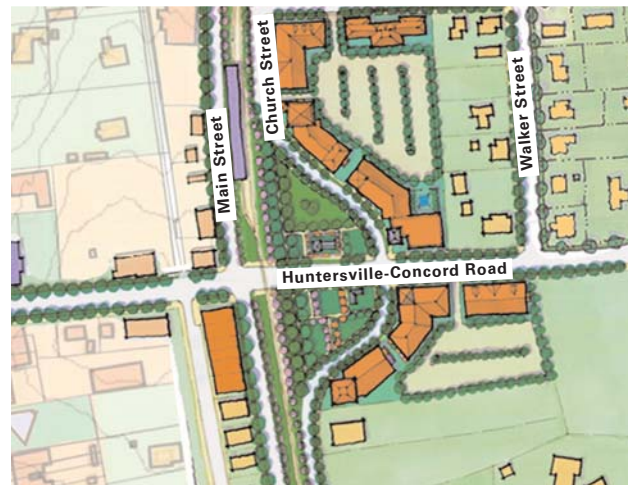
DESIGN PROPOSAL Area Plan proposal for intersection of Church Street and Huntersville-Concord Road, to provide the required 200 foot separation from Main Street
