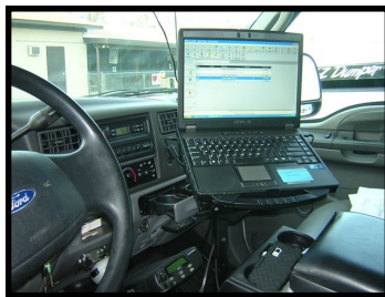
A newly installed MDT inside an Animal Control field officer's vehicle is pictured.
