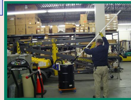
Building Maintenance’s “Bulb Eater” not only crushes old fluorescent lamps into 100% recyclable material, but also captures over 99.9% of the toxic vapors released.
